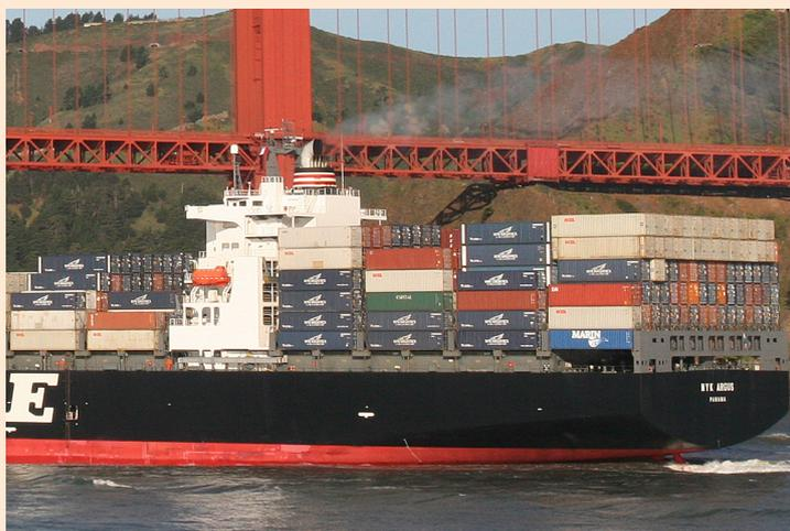
Specially designed MARIN measurement container (right bottom) on the NYK Argos
