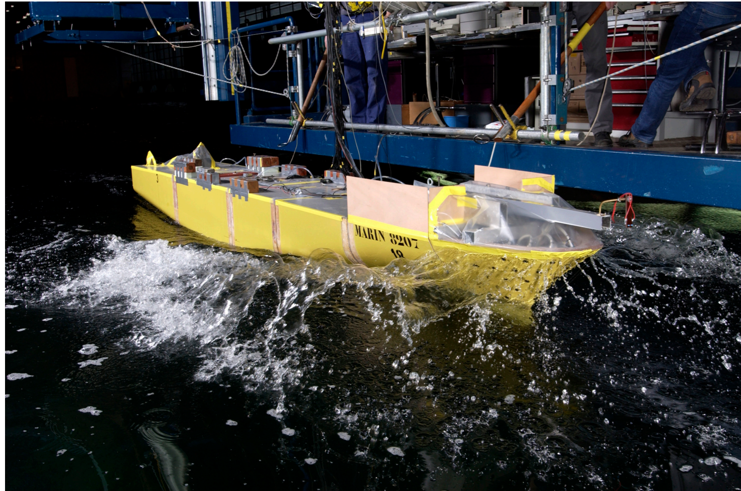
Segmented model with flexible beam (ELAST project)
