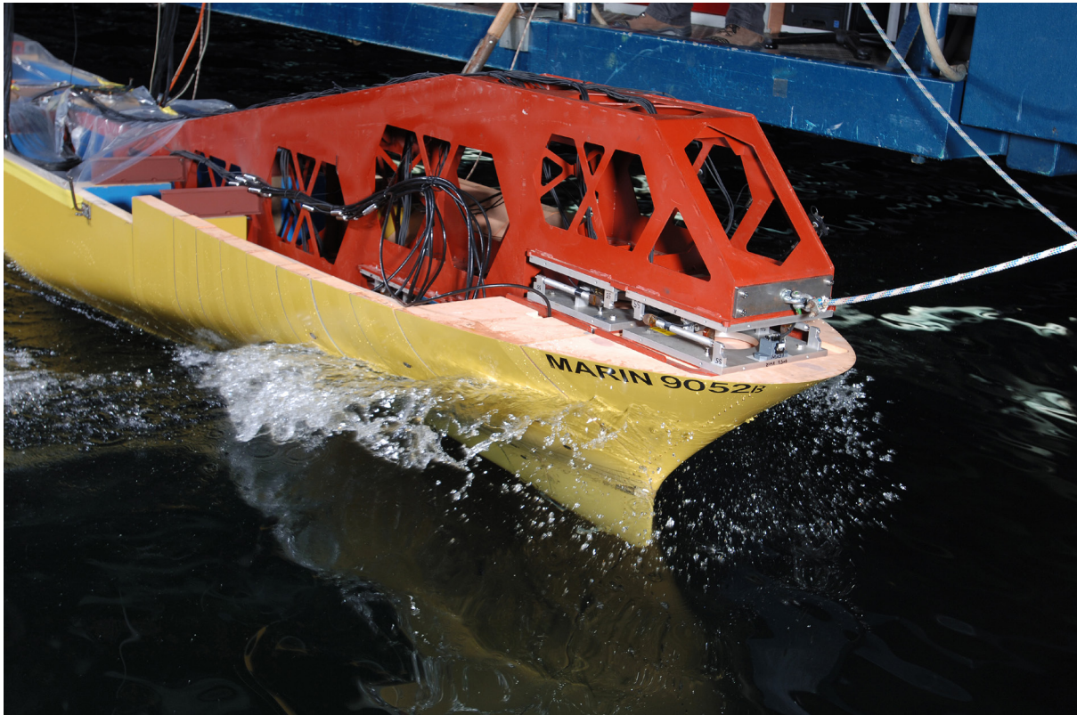
Free running experiments with a model having 10 segments in the bow area (WHIP-2 project)
