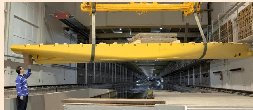
To measure the crabbing performance, large models need to be used. The model on the photograph was the CRS base model for many crabbing tests in deep and shallow water
