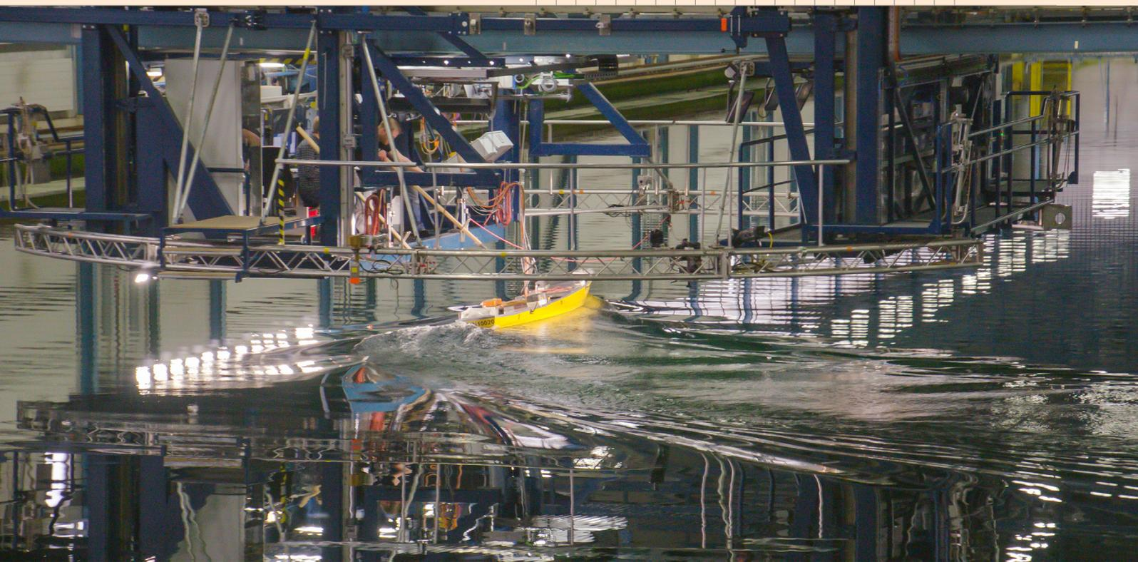
Acceleration turn in Seakeeping and Manoeuvring Basin (MORE project)
